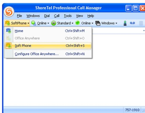
Figure 7-1 Activating SoftPhone from the Extension bar
